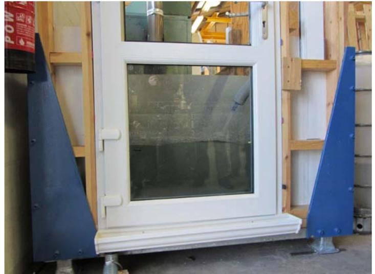
Photo above shows a flood resistant door under test. To see a door being tested go to <http://www.youtube.com/watch?gl=GB&v=iYAO7KaEO5k>
